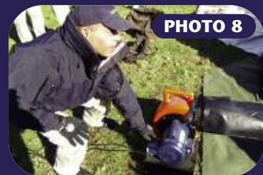
The interior bladder is inflated by a small, portable blower to raise the shelter.
